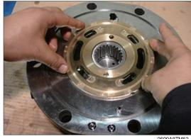
(8) Apply grease to the O-ring and then assemble O-ring into rear cover (34).
