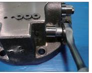
(4) Assemble relief valve (42, 2EA) into rear cover (34).
