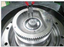
(13) Disassemble trust block (4) and oil-seal (3) into casing (1).
