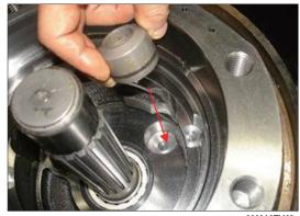
(18) Apply the grease to steel ball(15) and then assemble steel ball(15) into casing(1).
