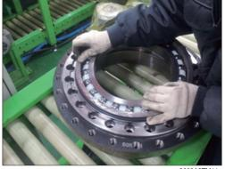
2 Release 25 hex wrench bolts (28. M18) and remove ring gear (1) from housing (7).
