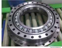
(2) Insert angular bearing (2) into reversed housing (7) on the same way.
