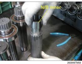
(12) Assemble snap ring (13) into Shaft (8) using pliers.
